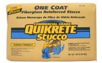
• QUIKRETE<sup>®</sup> One Coat FRS Concentrated is packaged in 80 lb (36.3 Kg) bags and must be field mixed with properly graded plaster sand in accordance with ASTM C897. Each 80 lb (36.3 Kg) bag should be mixed with approximately 210 lb (95.3 Kg) of sand.
