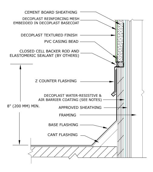
DCBS R1.02 CEMENT BOARD STUCCO - HIGH WALL AT LOW ROOF
