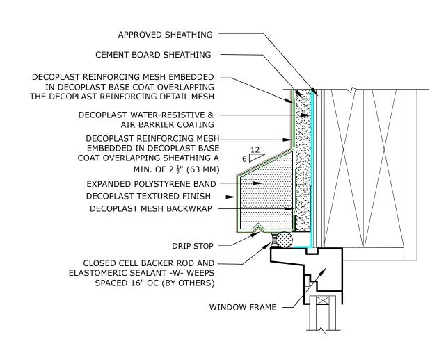
DCBS W1.02 CEMENT BOARD STUCCO - DECORATIVE BAND AT WINDOW HEAD DECOPLAST CEMENT BOARD STUCCO - 6/1/2016 NOTE:
