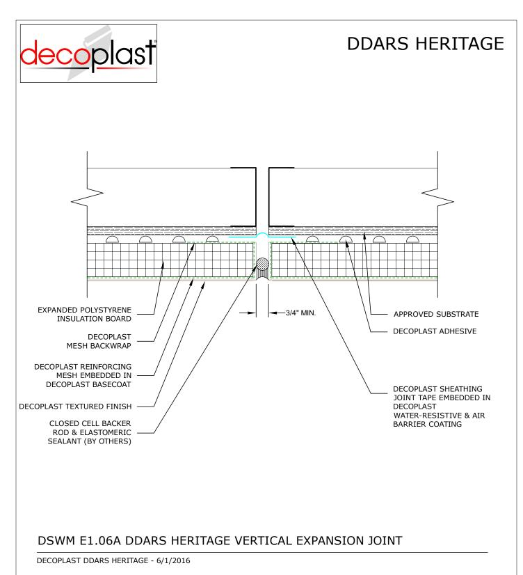
NOTE: To ensure a continuous air barrier across the building envelope, a continuous air seal should be made at each substrate change, joints/gaps, penetrations and dissimilar material terminations. These must be a consideration of the designer in the overall wall assembly design.
